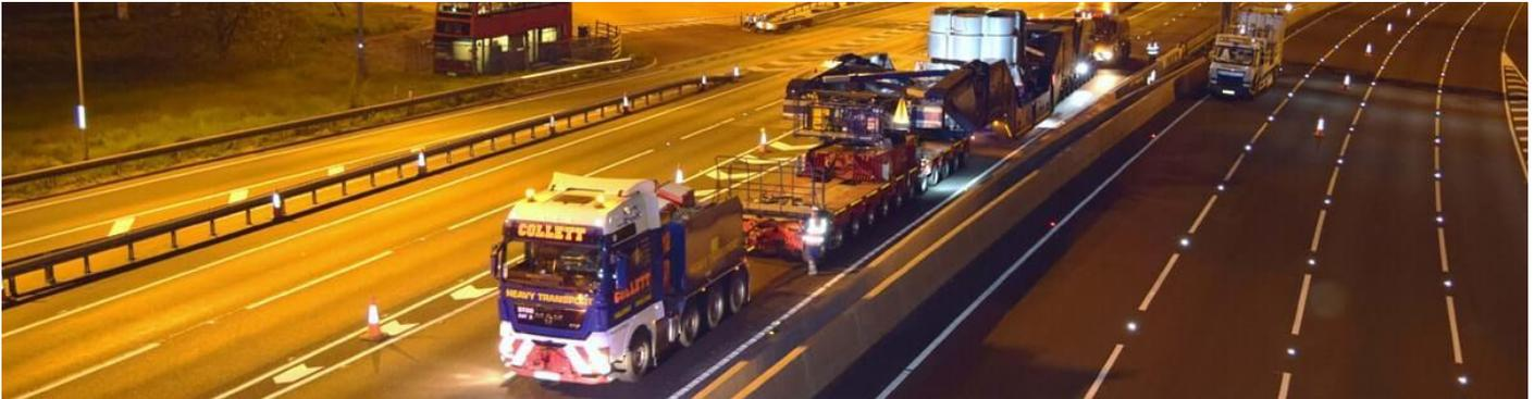
Following a similar successful operation in 2014 which required the relocation of six transformers, the project called upon the expertise of Collett to devise a solution for transporting each of the transformers, measuring 5.08m (H) x 3.5m (W) x 6.5m (L), from Dartford to Drax Power Station near Selby, North Yorkshire. Faced with the task of moving several abnormal loads originating within the busy capital the Collett Team began devising intricate transport arrangements to facilitate the loads.
