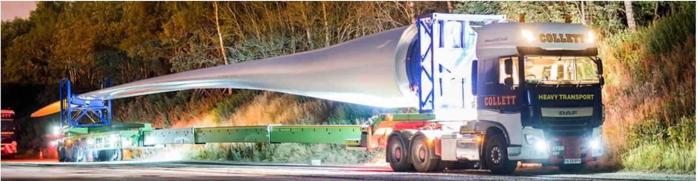
Our Teams undertook the planning and delivery of 494 components including blades, towers, nacelles, drive trains and hubs required for the development of Kype Muir Wind Farm. The 80m hub height towers of the Senvion 3.4MW turbines feature 52m blades, and whilst these are not the largest we've been appointed to handle, they necessitated the use of our Super Wing Carriers due to the problematic road restrictions and alignments en-route.
