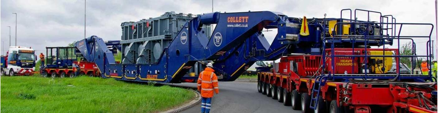
With the transformer arriving at Port Sutton Bridge our Team carried out all port services including stevedoring, lift plans, crane hire and CPA Contract Lift by mobile crane, discharging the 8.6m L x 4.91m W x 4.75m H cargo from the hold of the vessel to our Scheuerle girder bridge.
