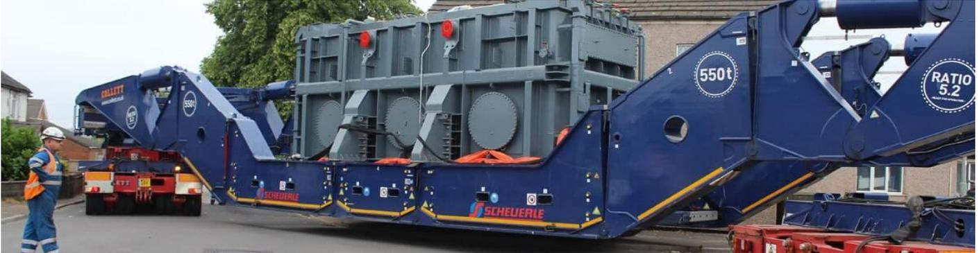
Loaded to a specialist 550 Tonne capacity Scheuerle girder bridge, and accompanied by two heavy tractor units in push/pull formation, the 69.6m long combination travelled the 67 miles from Ellesmere Port to Cellarhead Substation in Stoke-on-Trent.
